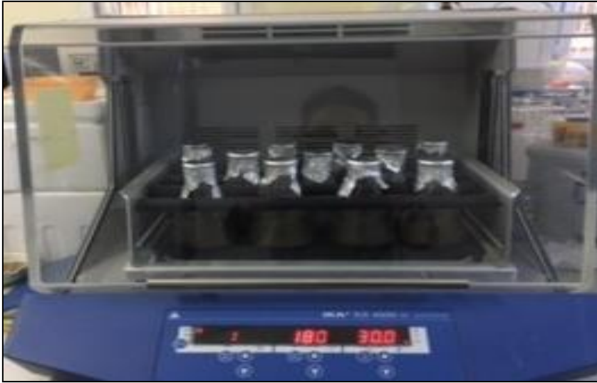
Figure 2.4. Bioleaching experiments performed in incubator shaker
