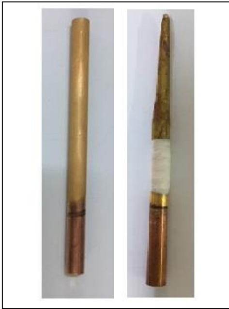
Figure 3.45. Gold coated copper electrodes at the anode part before and after the electro dialysis (left side: before electro dialysis, right side: after electro dialysis)
