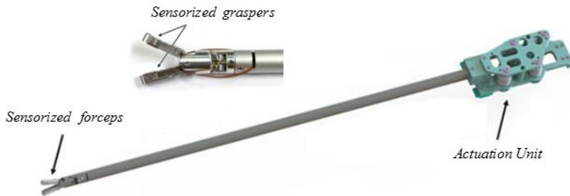
Figure 1.4. 4-DOF sensorized instrument including Raven 2 adapter
