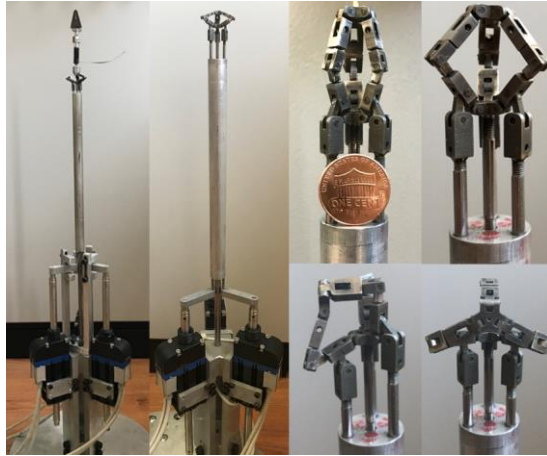
Figure 2.2. Forceps mechanisms with and without a gripper
