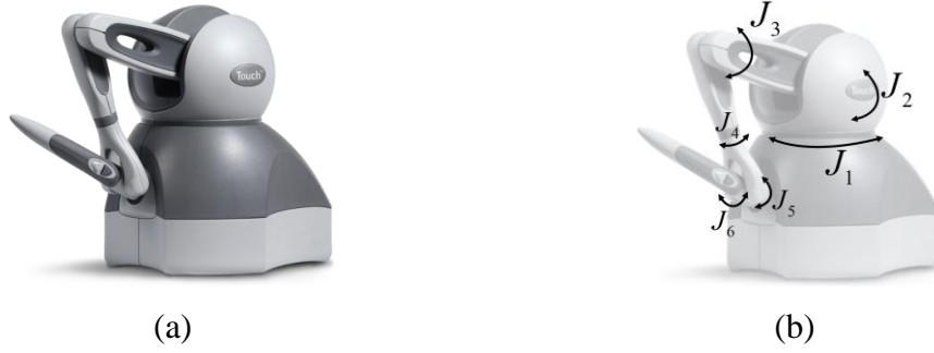
Figure 6.2. Phantom Omni robot (a) General view (b) Representation of joints
