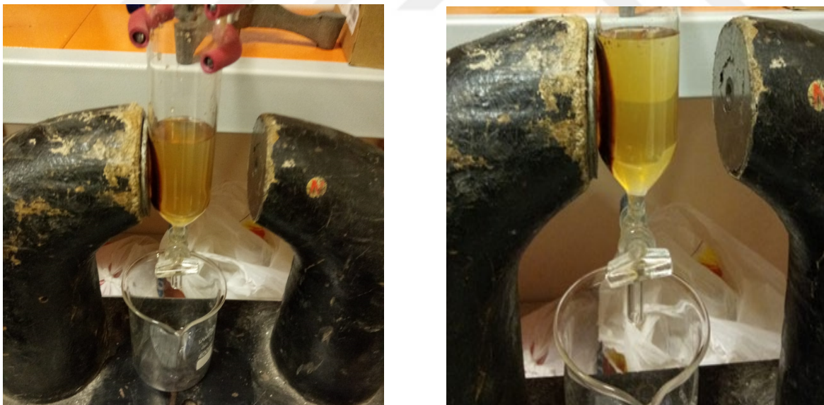
Figure 3.5 Collecting Nanoparticles with Magnet
