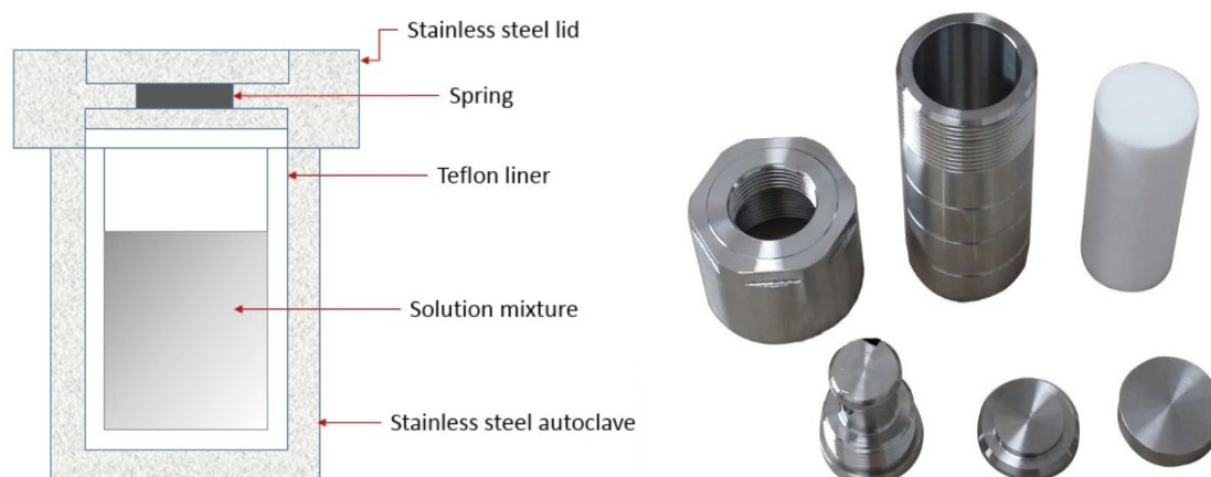
Figure 2.2 Crosssectional view and components of the autoclave.
