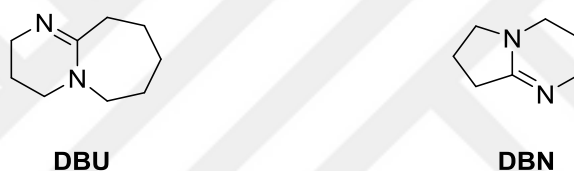
Figure 2.4. Structures of 1,8-diazabicyclo [5.4.0] undec-7-ene (DBU) and 1,5-diazabicyclo [4.3.0] non-5-ene (DBN)
