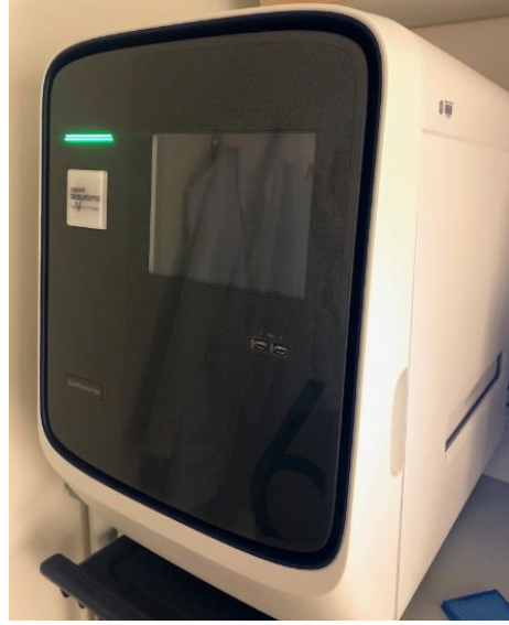
Resim 9: Real Time Machine (ABI Prism QuantStudio 6 Flex, Applied Biosystems, Foster City, CA) Cihazı
