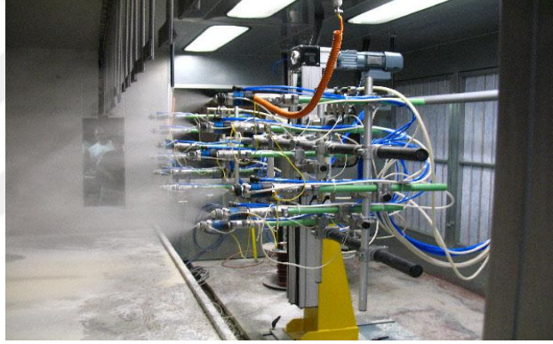
Şekil 3.7. ESTA uygulama kabini (Referans: https://www.eic-vitreous-enamel.com/equipment-process/coating/spraying/electrostatic-wet-enameling.html , 2019)
