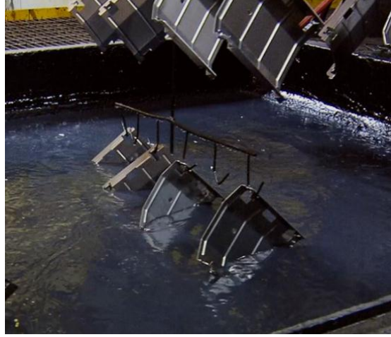
Şekil 3.9. Elektroforetik emaye kaplama hattı (Referans: http://www.ferrotechnikcolombia.com.co/enamelling-technology/epd-electrophoretic-deposition , 2019)
