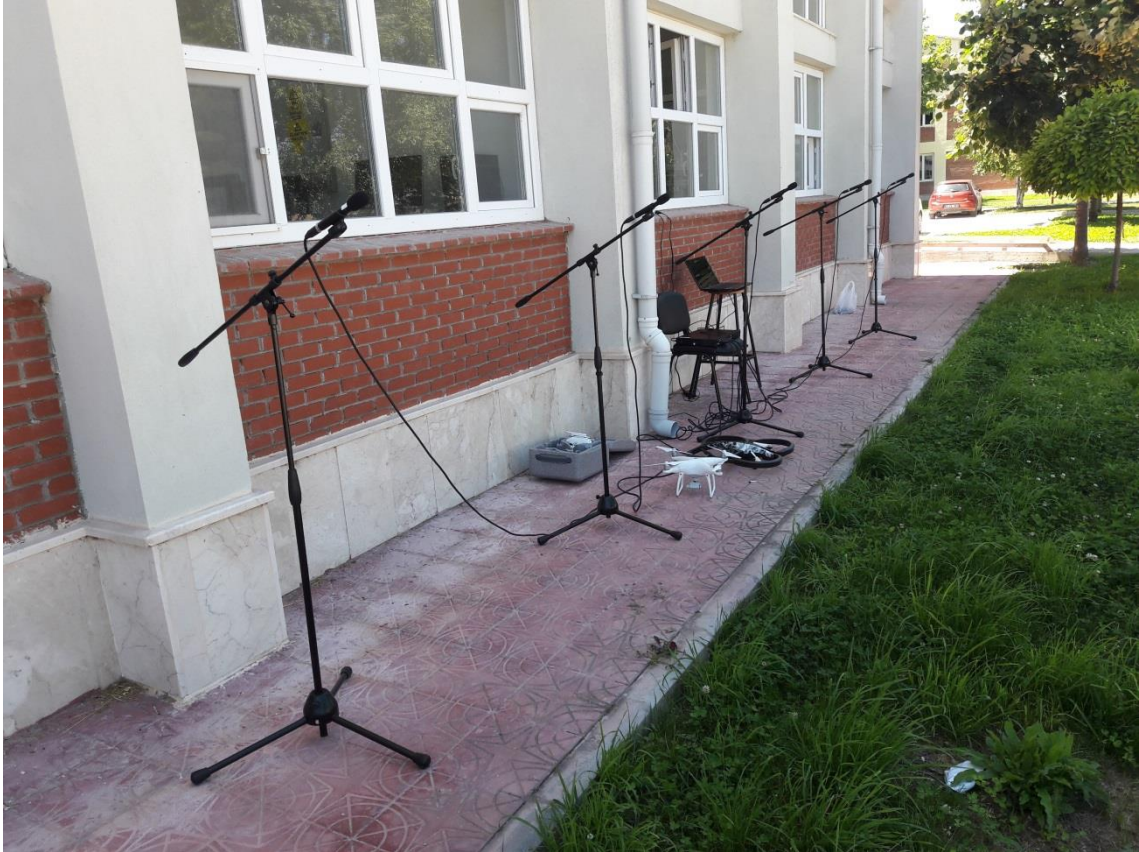
Figure 4.24. Installing an array of 5 AT2031 microphones with US1800 sound card
