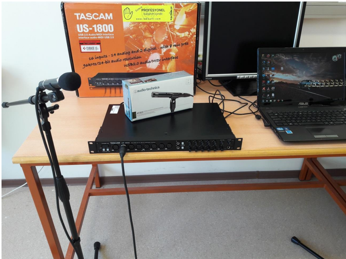
Figure 4.23. The hardware tools US-1800 and AT2031
