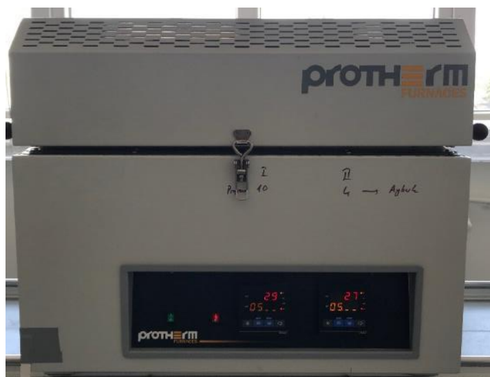
Figure 3-3 Chemical vapor deposition system two heat zoned furnace
