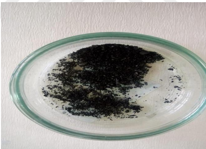
Figure 3.1. Homogenous carbon paste mixture containing 0.3 g of graphite powder, 0.076 g of modifier material (FS@Ag) and 150 \mu L nujol oil
