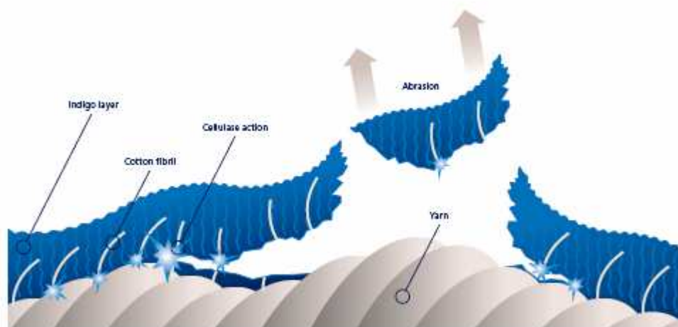
Figure 1.8: Stone washing effect of cellulases on denim fabric [49].
