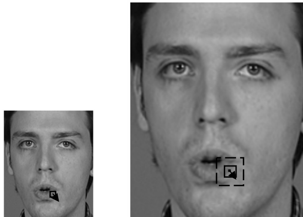
Figure 4.7. Illustration of the displacement estimation algorithm. Motion vector found in bilinearly interpolated face frame (right), and motion vector of the corresponding block in the original frame (left).
