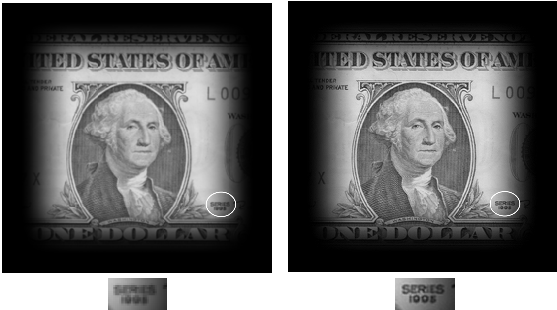
Figure 3.3. Result of bilinearly interpolating a LR dollar image by a factor of two (left), and result of superresolution algorithm with pixel-domain POCS method using 4 LR images (right).
