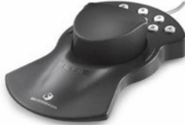
Figure 5.7. Magellan space mouse used for simulation
