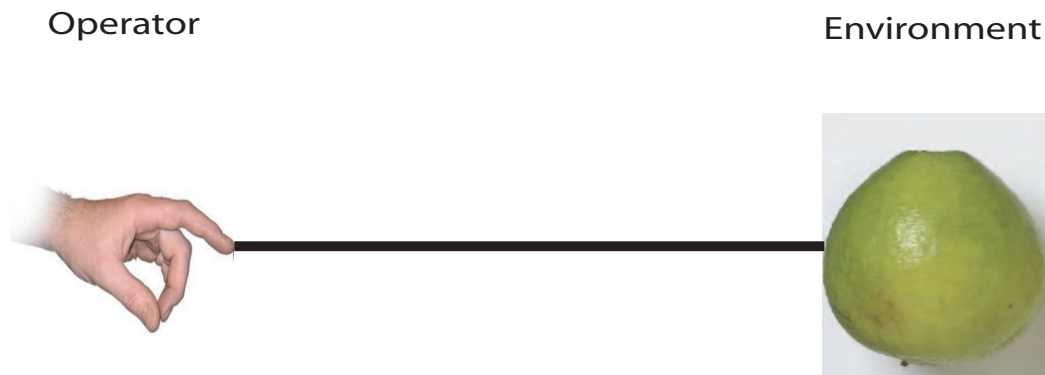
Figure 2.6: Rigid coupled ideal bilateral teleoperation system, adapted from [5]
