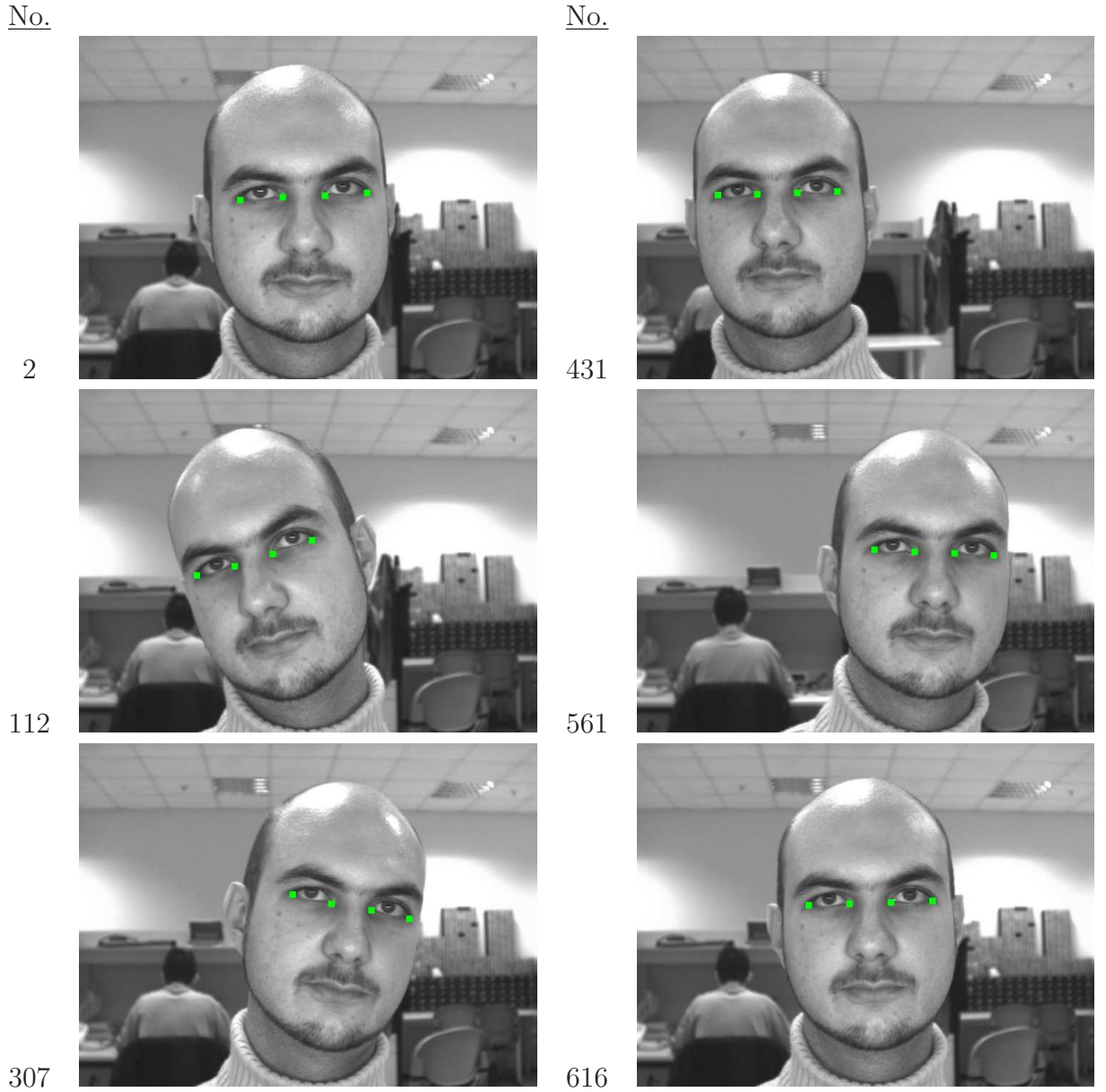
Figure 4.2: Tracking results of the proposed method for a sequence that includes head rotation around z-axis and translation in x-axis.
