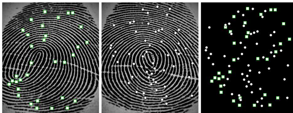
Figure 3.3: Two fingerprints A (on the left) and B (in the middle) are combined to form the multi-biometric template ( A \cup B on the right). Minutiae points are differently marked for the sake of clarity.
