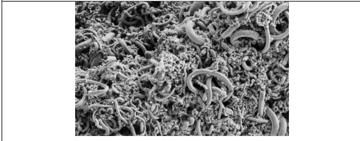
Figure 3.14 The voltammogram of CNF templated PPy deposited via 6 times cycling at a scan rate of 200 mV/s, and its SEM images: (b) 20000 times magnified (c) 50000 times magnified.
