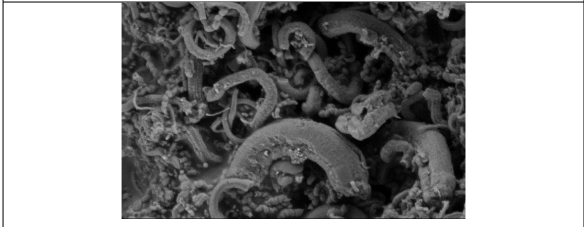
Figure 3.13 The voltammogram of CNF templated PPy deposited via 7 times cycling at a scan rate of 150 mV/s, and its SEM images: (b) 20000 times magnified (c) 50000 times magnified.
