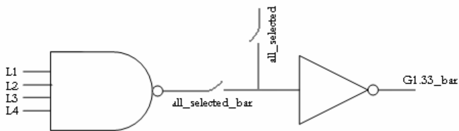
Figure 3.15: Digital logic to set automatic gain adjustment control signal, G1.33_bar
