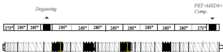
Figure 3.1- Temperature profile of the co-rotating intermeshing twin screw extruder.
