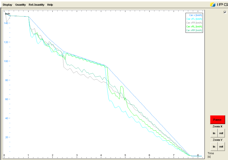
FIGURE 4.25: WHEEL & VEHICLE VELOCITIES (SCENARIO IV, SMC-ABS, 50°)
