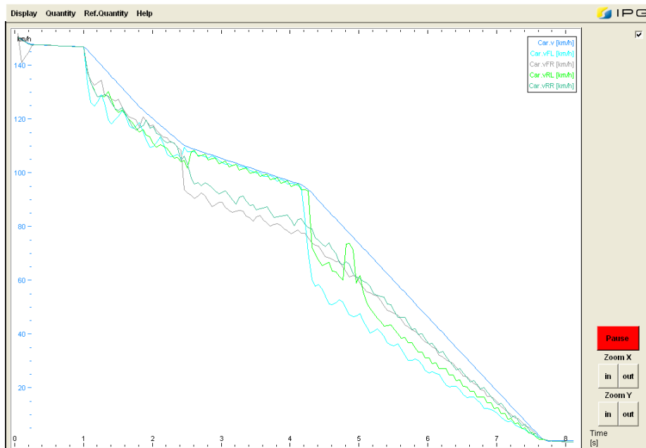
FIGURE 4.19: WHEEL & VEHICLE VELOCITIES (SCENARIO IV, SMC-ABS, 360°)
