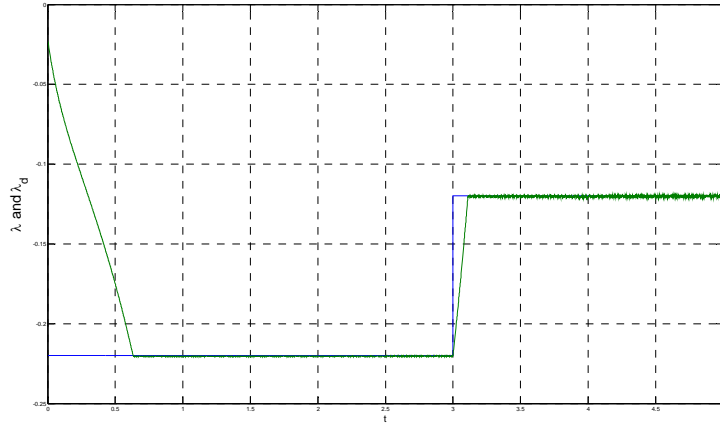
FIGURE 3.11: \lambda VS \lambda_d (SMC SLIP CONTROLLER- TRACKING, W/O T_E )
