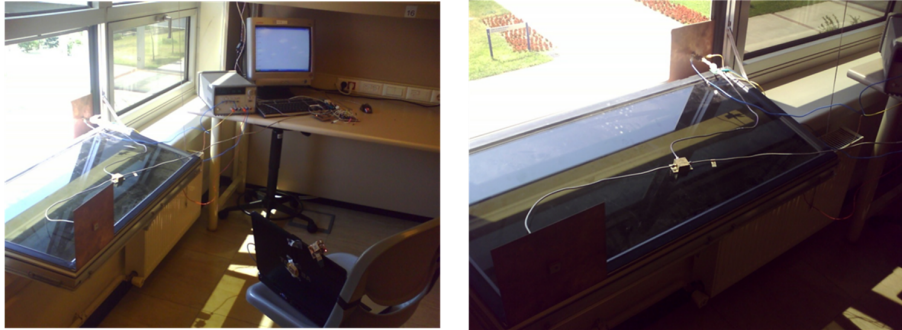
Figure 3.30: Measurement setup for path loss measurements with GPS receiver
