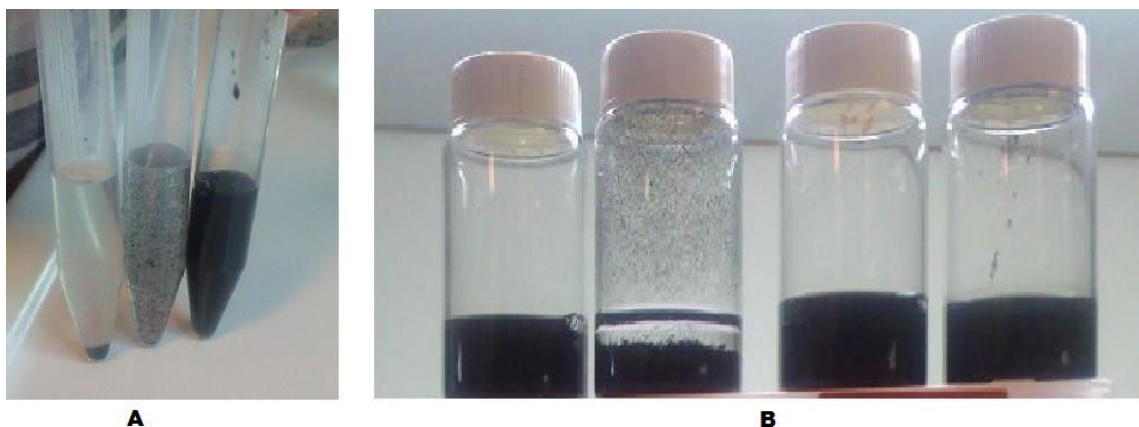
Fig 4.1. Dispersion of MWNTs. (A) MWNT_COOH in ddH 2 O with no treatment (left), MWNT_COOH + Triton 100X (middle), MWNT_COOH + Triton 100X + Sonication (right). (B) MWNT_NHS in ddH 2 O, MWNT_APTES in EtOH, MWNT_COOH in ddH 2 O, MWNT_OH in ddH 2 O, from left to right, respectively.
