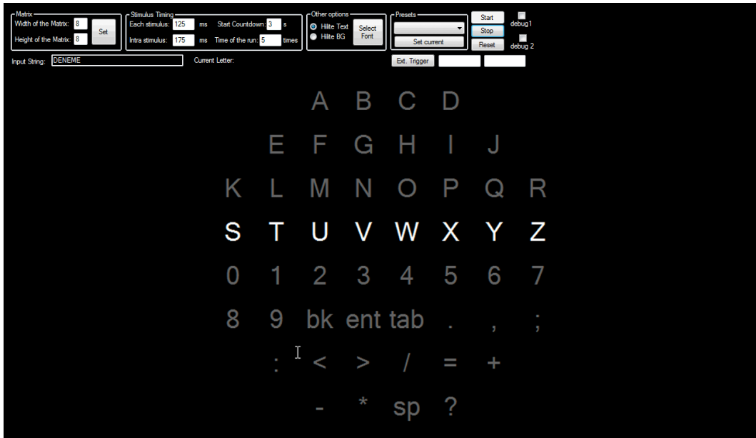
Figure 3.3 A round matrix. Although the matrix is 8x8, some elements at each corner are left blank to get a “round” shape.
