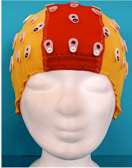
Figure 2.1 64-channel electrode cap featuring international 10-20 system for electrode distribution [7]
