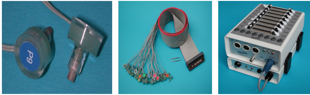
(a) Active Electrodes (b) Electrode Bundle with 32 Electrodes (c) Biosemi Active 2 Amplifier and Battery
