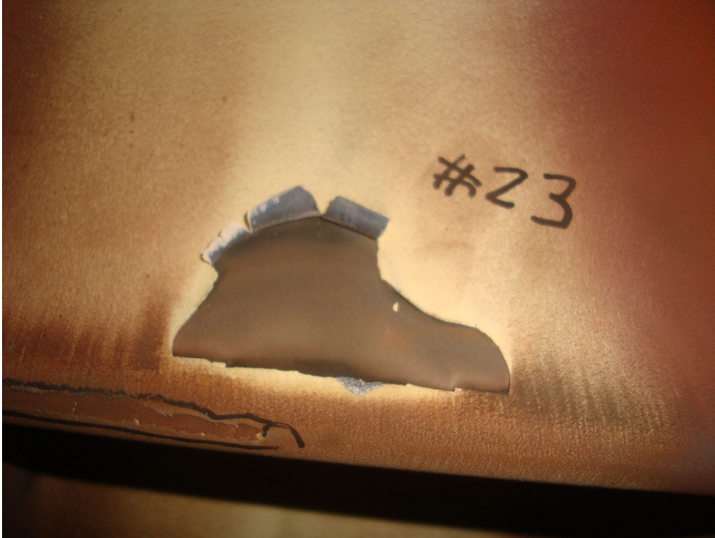
Figure 28: Worn Turbine Vane Coating
