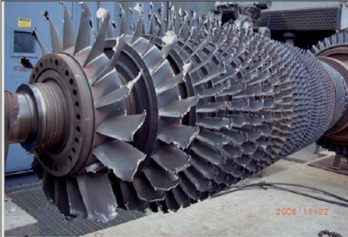
Figure 27: Catastrophic Failure of a Gas Turbine
