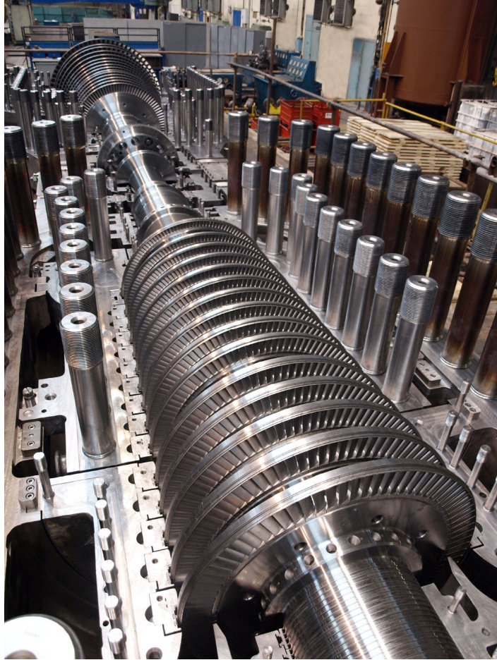
Figure 16: HP and IP Sections of a Steam Turbine ( www.skoda.cz )
