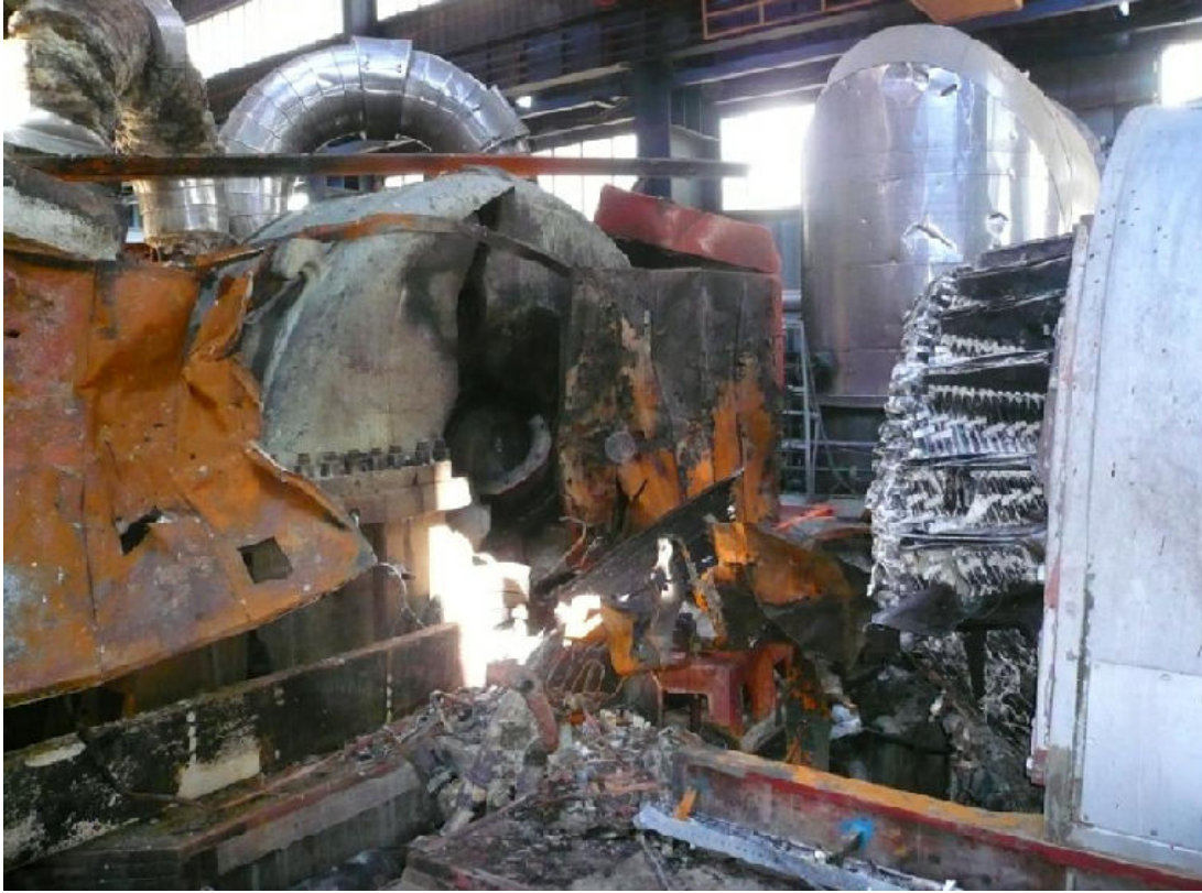
Figure 48: A Disastrous Failure of a Steam Turbine & Generator ( www.steamforum.com )
