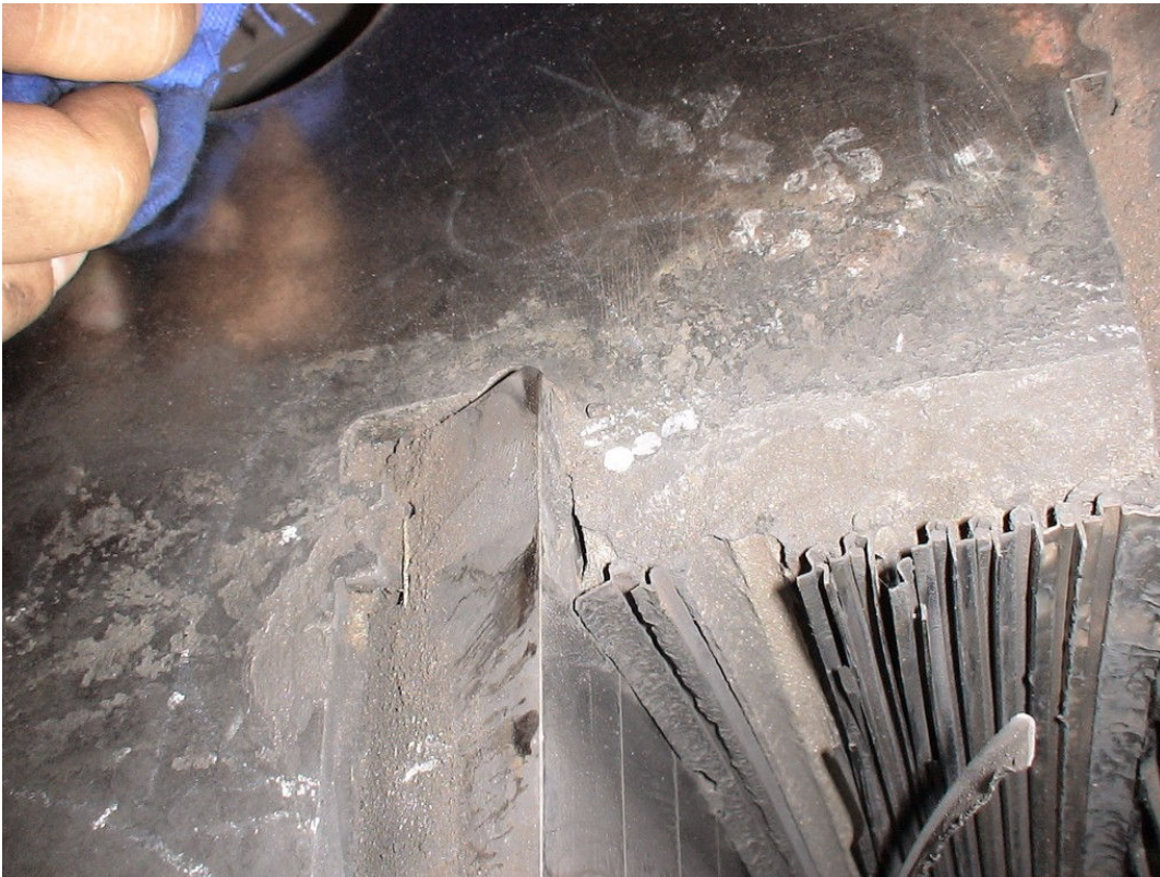
Figure 36: Worn Labyrinth Seals
