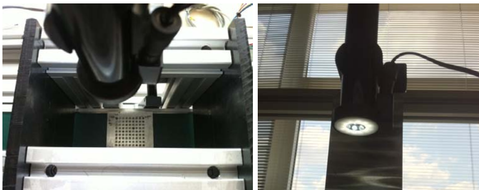
Figure 6-89 – (a) Vision Station (b) Ring Light
