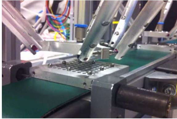
Figure 6-99 – Two Delta Robots Realizing the Assembly Operation Simultaneously
