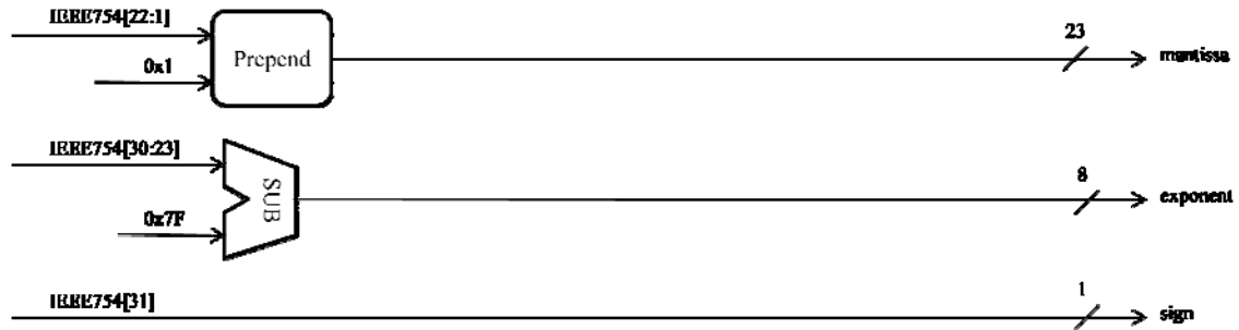
Figure 3.3: Block structure of from IEEE754 standard to EFP conversion unit.
