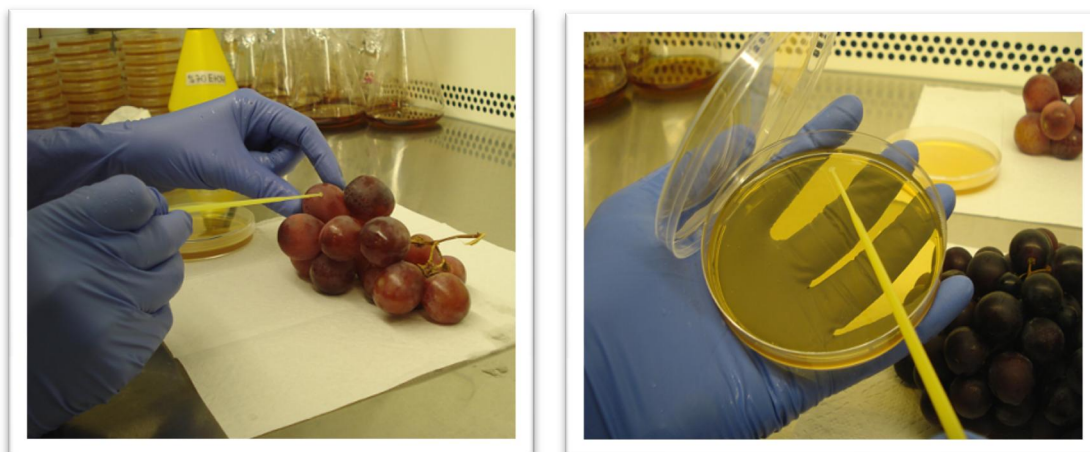
Figure 11 Representation of streaking method from one berry.
