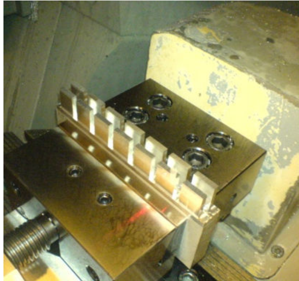
Figure 3-10 Flexible workpiece setup
