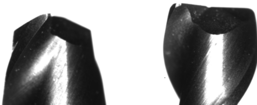
Figure 4-3 Chipped edge of a test tool
