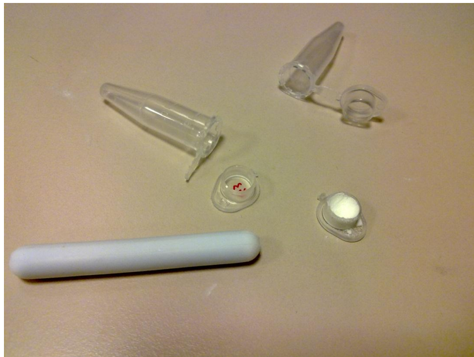
Figure 2.2 Lids of the eppendorf tubes are cut and filled with the \text{SA}_2 powder. Then the powder is pressed with the help of a magnetic stirrer.
