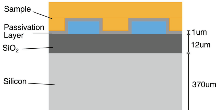
Figure 25: Capacitor structure that is used for simulating capacitance change of W: 2.5\mu\text{m} -G: 5\mu\text{m} structure using Coventorware FEM tool
