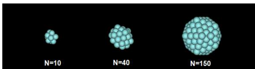
Figure 2.4. Atomic configurations of the nanoclusters of different sizes ( N=10, 40, 150 )
