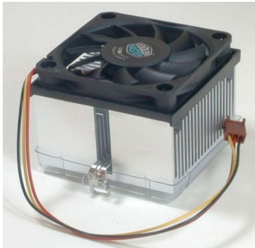
Figure 1.1. CPU cooling with a heat sink and a fan [3].
