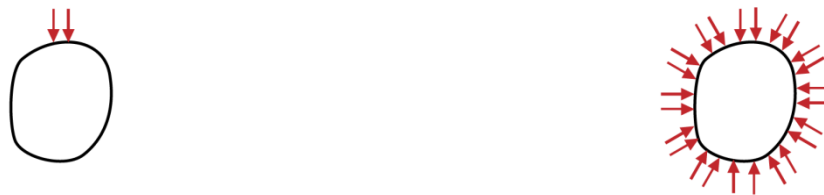
Figure 15 (a) Erosion in bubble path direction for stationary sample (b) Erosion in every direction for rotating sample
