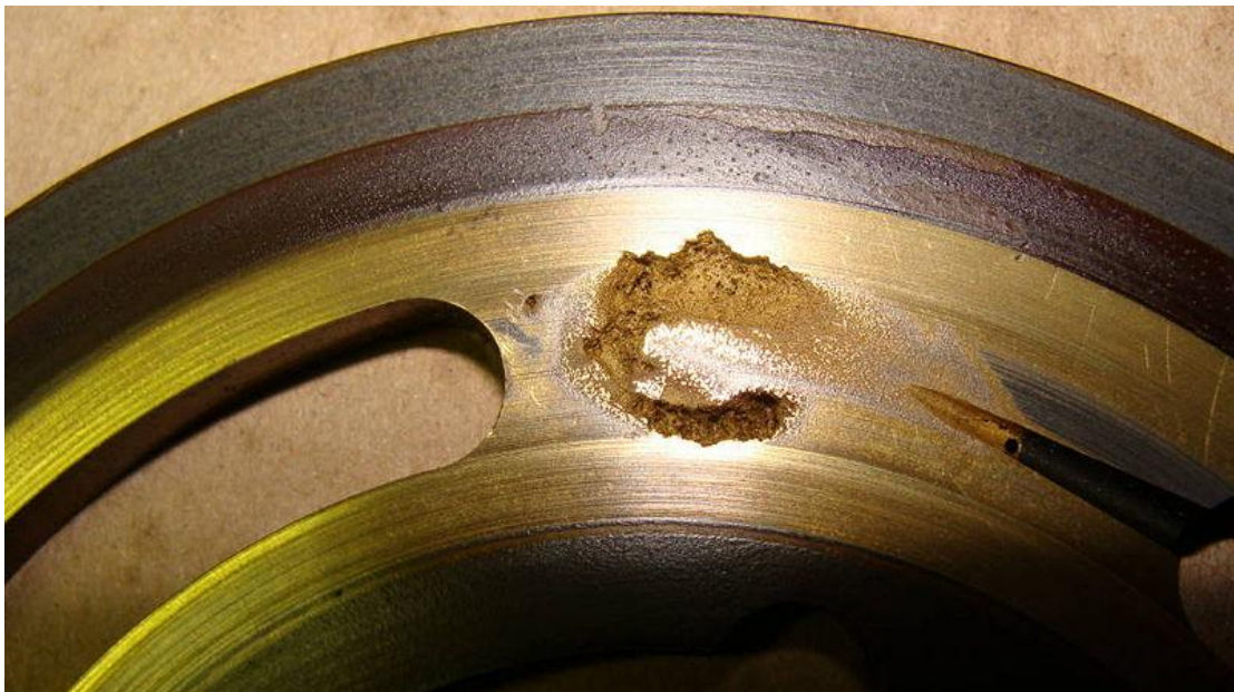
Figure 1 Cavitation damage on a valve plate for an axial piston hydraulic pump [2].
