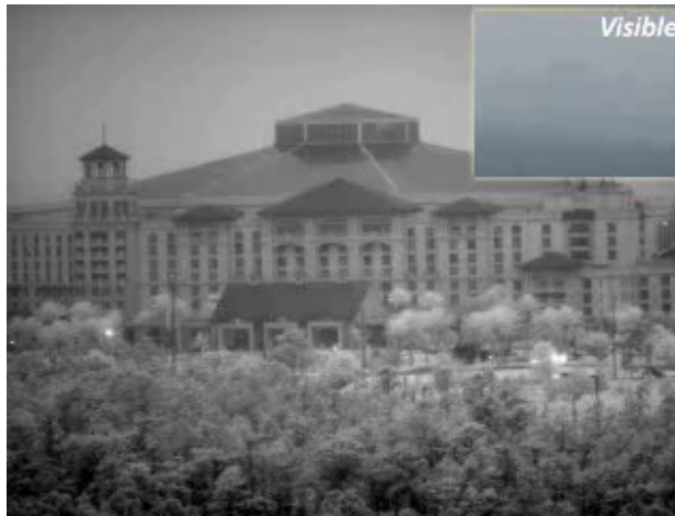
Figure 8. Imagery taken with a SWIR camera of a hotel from more than a mile away in the midst of haze. Frame on the top right is the same hotel and weather conditions imaged with a commercial visible camera [21].
