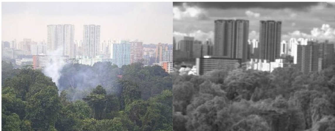
Figure 7. Building scene in the presence of fog recorded by visible camera (on the left) and by a SWIR camera [20].
