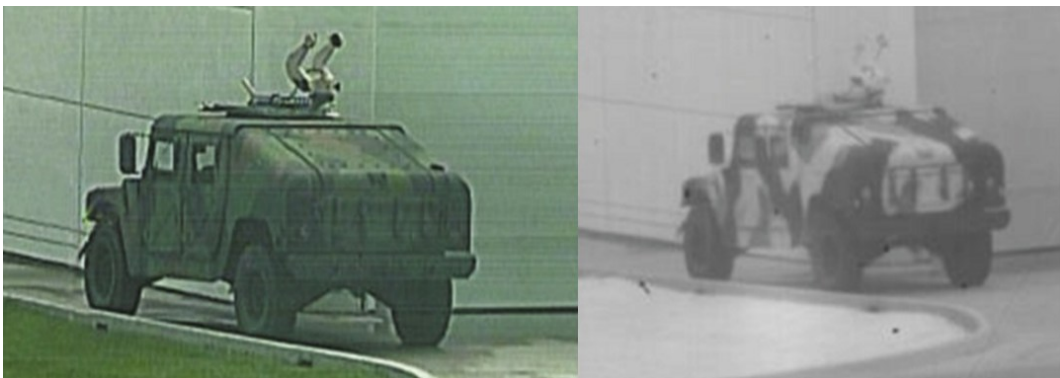
Figure 6. Visible (left) and SWIR (right) image of a Humvee. In SWIR, the camouflage is less effective [19].
