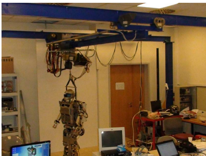
Figure 4.50 : SURALP, research laboratory and Cartesian crane system
