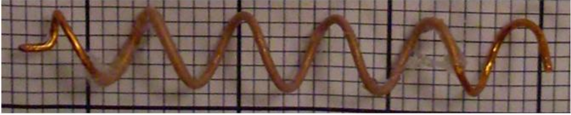
Figure A6.20: Tail with \lambda = 12 mm; B_o = 4.5 mm; L_{tail} = 60 mm.
