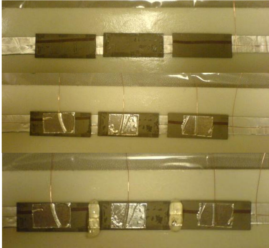
Figure A1.15: Experimental piezo-strip: All bender piezo-ceramic stacks are placed on a common ground, separate power leads are included and secured, and piezo-ceramic stacks are rigidly linked together with hot silicon, which is an electric insulator.
