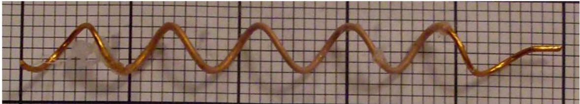
Figure A6.19: Tail with \lambda = 16 mm; B_o = 4.5 mm; L_{tail} = 93 mm.
