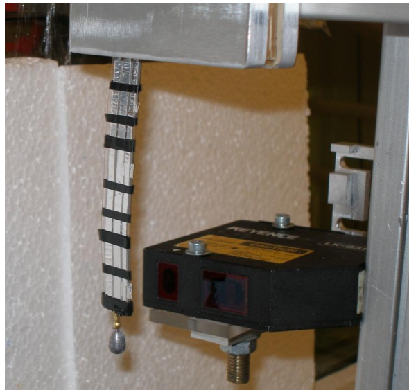
Figure A1.16: Experimental (displacement sensing) setup: Orientations and positions of the piezo-strip and laser displacement sensor.
