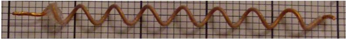
Figure A6.18: Tail with \lambda = 10 mm; B_o = 2.5 mm; L_{tail} = 88 mm.
