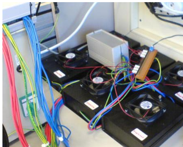
Figure A1.11: Picture of protective boxes with high-voltage-amplifier board installed (6 channels in total).
