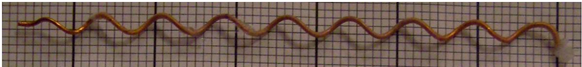
Figure A6.17: Tail with \lambda = 15.5 mm; B_o = 2.5 mm; L_{tail} = 130 mm.
