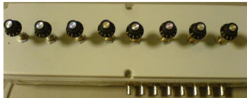
Figure A1.8: Picture of the assembled 8 channel analog signal control box and tuning knobs.
