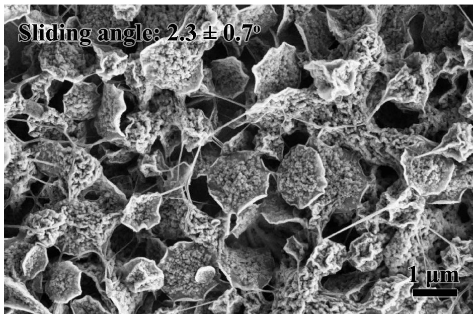
Figure A.7: Typical SEM image of the electrospayed surfaces from 1.5 wt% poly(st- co -PFA) solutions in 50/50 (wt/wt) THF/NMP mixture (8 kV applied voltage and 0.5 \mu\text{L}/\text{min} solution feed rate).
