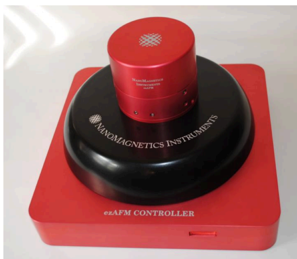
Figure 4.3: Latest Generation ezAFM Electronic Controller, Vibration Isolation System and ezAFM Head Unit
