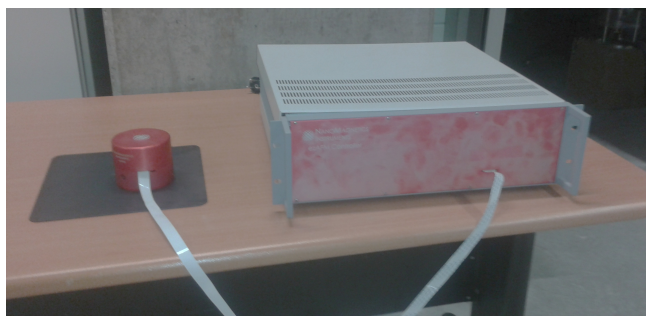
Figure 4.1: First Generation ezAFM Control Electronics and the Head Unit
