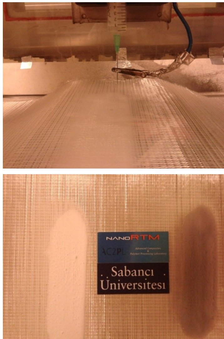
Figure 4.8. Electrospinning of Poly[co-GMA-Styrene] on the glass fiber layer(left) and electrospun Poly[co-GMA-Styrene] and CNT- Poly[co-GMA-Styrene] polymer mixture regions can be seen on [0/90] biaxial glass fabric(right).
