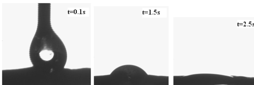
Figure 3.9. Frames taken during DSA measurements. Average contact angle is 26.5±6.10° for distilled epoxy droplet.
