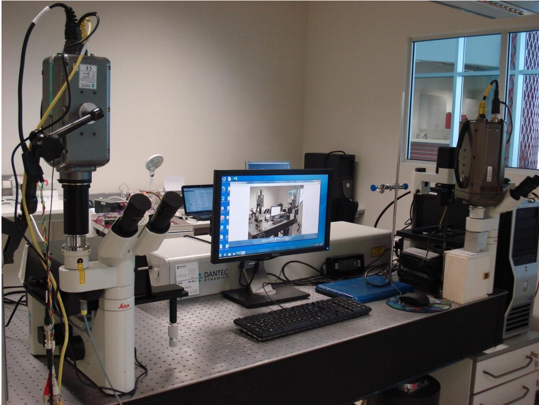
Figure 5.26 Double-frame micro-PIV imaging system consists of a cooling unit, a Neodymium-doped yttrium lithium fluoride (Nd:YLF) laser having a maximum output of 150W, a Phantom v130 high speed camera connected to Leica DMILM inverted microscope.
