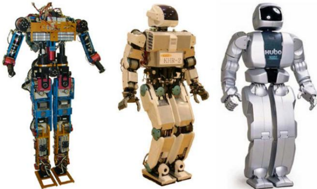
Figure 2.7 From left to right: KHR-1, KHR-2 and KHR-3 (also known as HUBO) [25-27]
