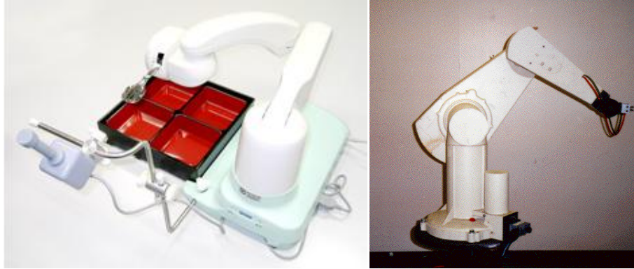
Figure 2.1 On the left MySpoon assistance robot, on the right puma 560 robot arm ([6] and [1])
