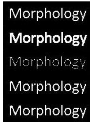
Figure 4.3 Common morphological operations. From top to bottom: original binary image, dilation, erosion, opening and closing operation.
