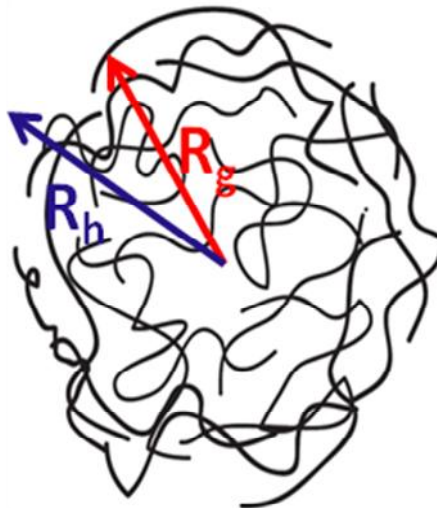
Figure 5: Schematic of the difference between hydrodynamic radius and radius of gyration.
