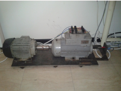
Figure 6-42 DFIG (on the right) coupled to wind turbine emulator (on the left)
