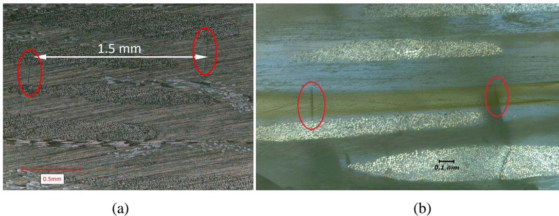
Figure 2.6: Microscopic images of cross section of specimens in loading directions. Transverse cracks just above the fiber optic cable (b) can be seen clearly. The cross section is taken along the fiber direction.
