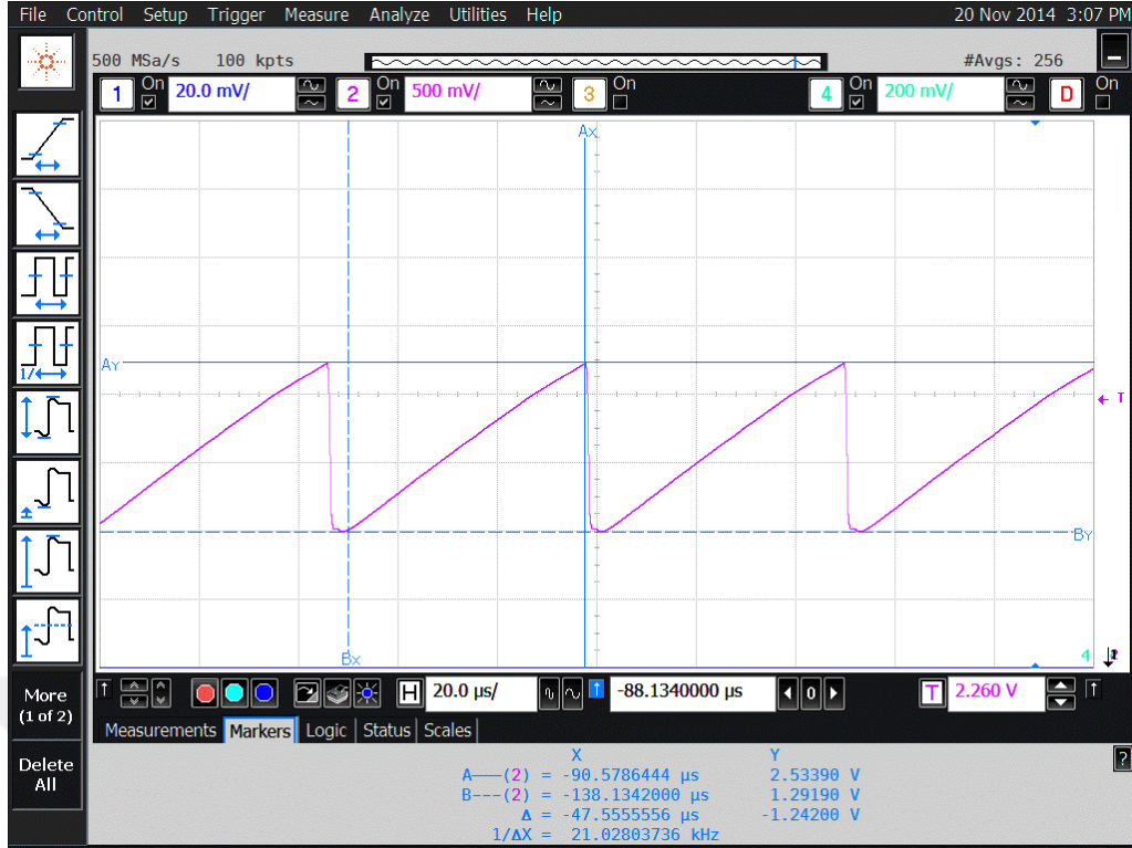
Figure 39: 50 \mu s integration time, 2.714V bias voltage, and 1.24V integrated charge.
