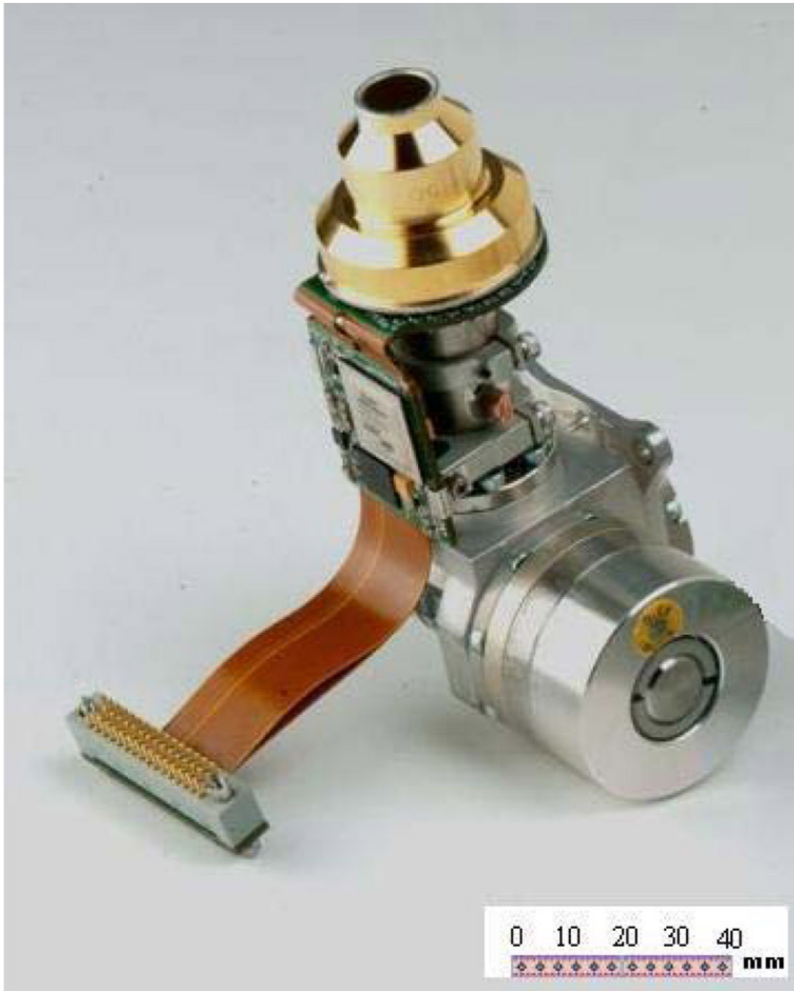
Figure 7: Cryogenic Dewar with Stirling cooler [21].
