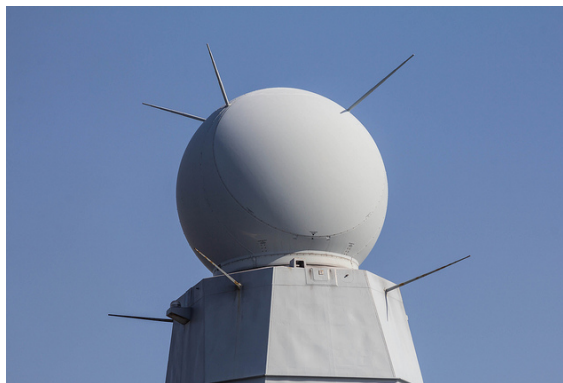
Figure 7: Active phased array example: SAMPSON[4]
