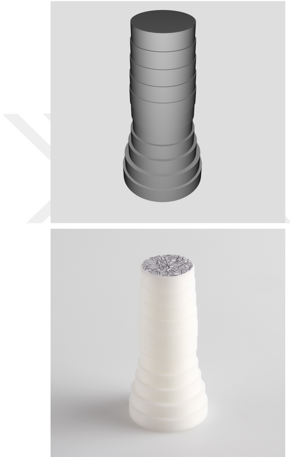
Figure 7.2: Generated 3D mesh and fabricated actual model
