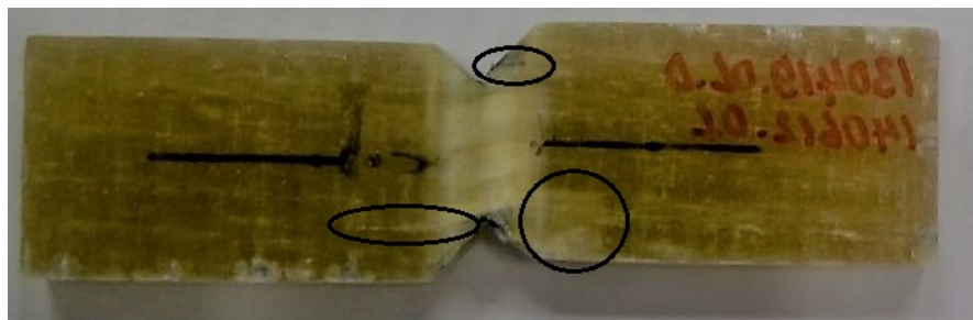
FIGURE 5.6: A tested Iosipescu shear specimen.
