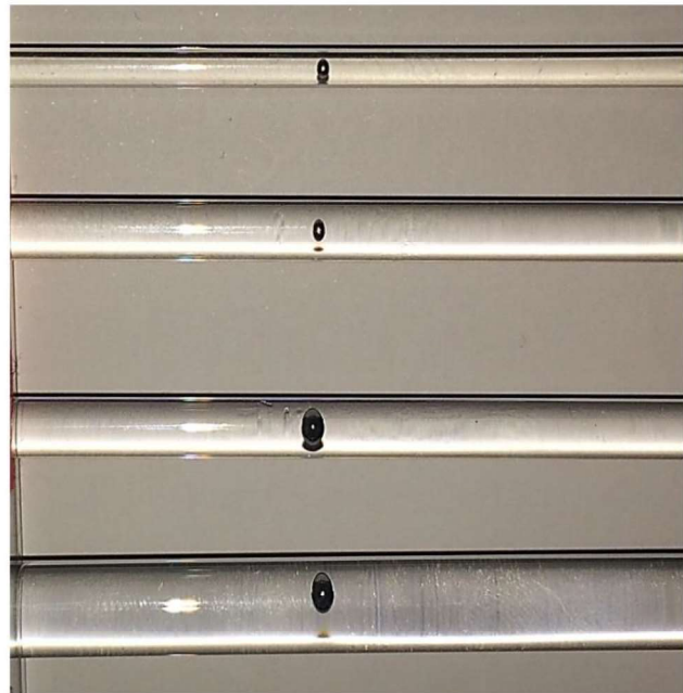
Figure 3.2 Cylindrical glass channels filled with silicone oil and magnetic spheres placed inside the channels.
